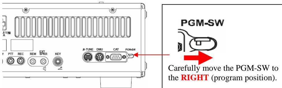
3. Connect the serial straight through programming cable, DB9F to DB9F, connector to the serial port COM1 in the back of your computer. Plug the DB9F connector to the CAT connector on the FT-950. If you use a USB to serial adapter, you might need to change the COM Port number.
